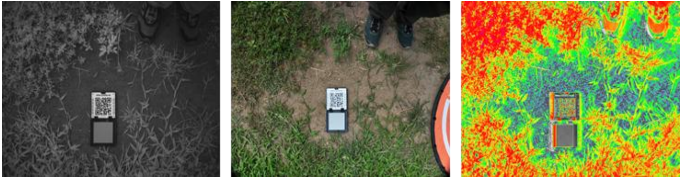
Figure 3. Micasense Calibrated Reflectance Panel (CRP) RP06-2123093-OB Source: Analysis results
